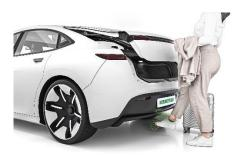
Enables opening and closing of sliding doors and trunks even with no free hand: The Hands Free Access Sensor by Schaeffler is activated by a foot movement – no button press or remote needed.
